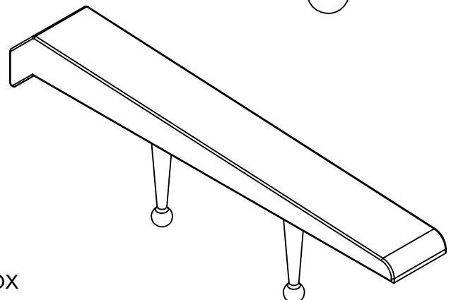
316 Stainless Steel surface mount. Drill and epoxy mounting pins into predrilled holes.
