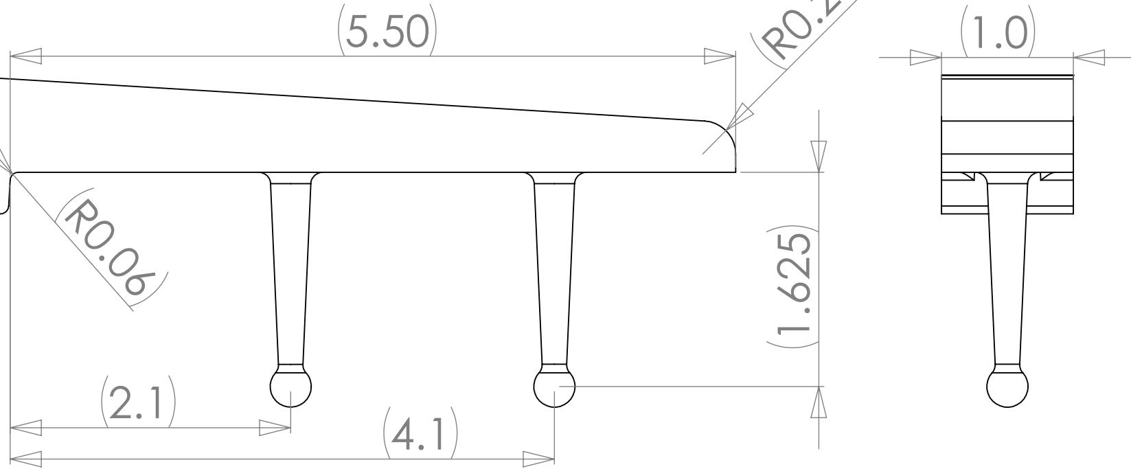
316 Stainless Steel surface mount. Drill and epoxy mounting pins into predrilled holes.
