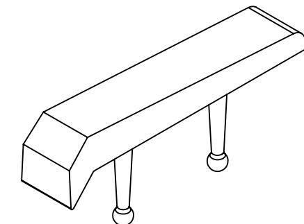
316 Stainless Steel surface mount. Drill and epoxy mounting pins into predrilled holes.
