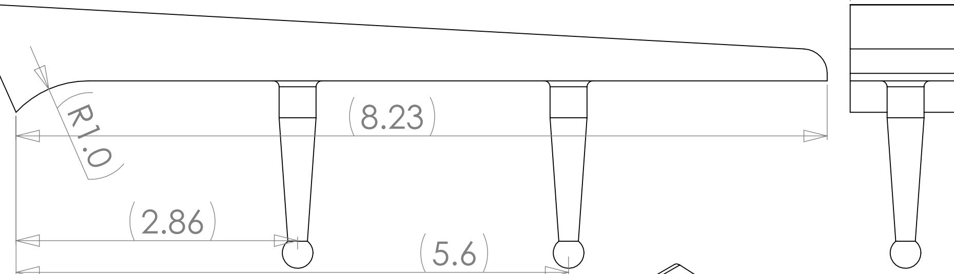
316 Stainless Steel surface mount. Drill and epoxy mounting pins into predrilled holes.
