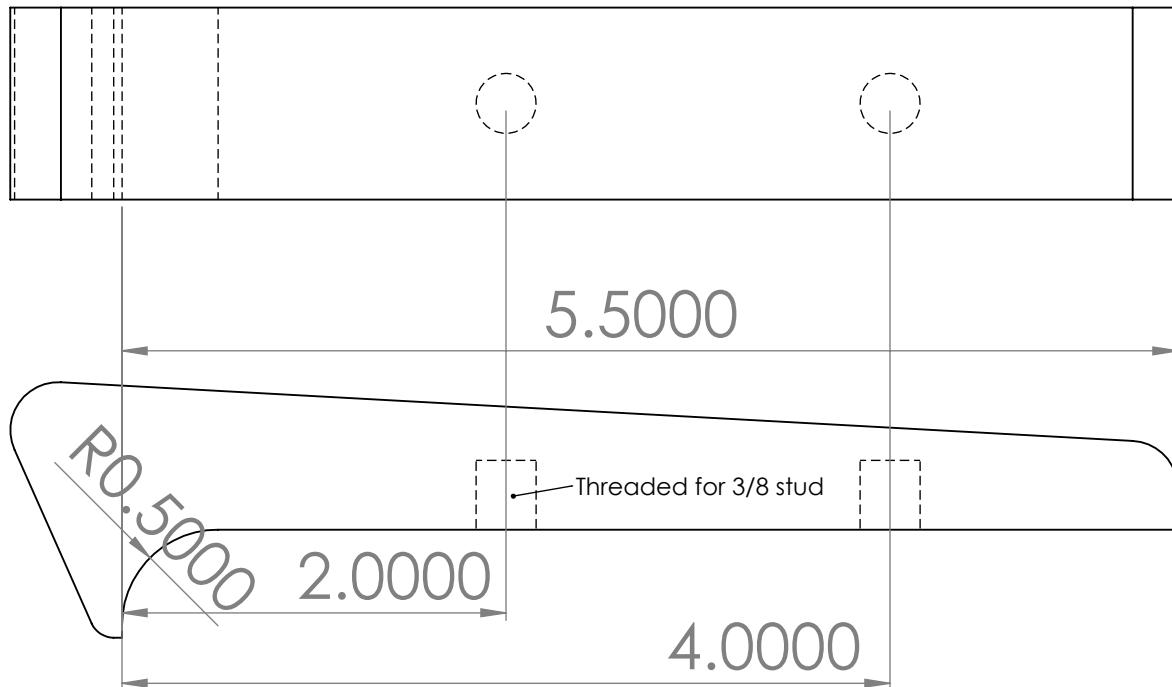
6061 T6 Aluminum. Deburr. Type II Clear anodize or Hard Anodize.
