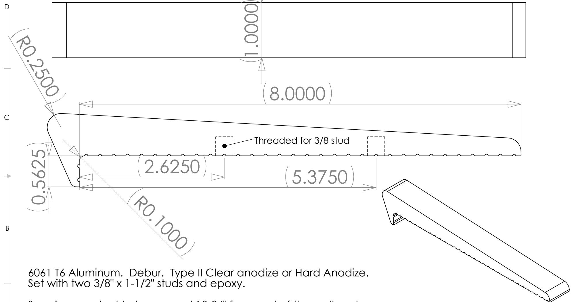
6061 T6 Aluminum. Debur. Type II Clear anodize or Hard Anodize.
